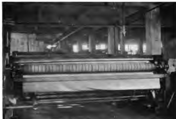
Fig. 2. Flat-Work Ironer with Guard over Rolls.
